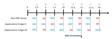
Note: where IS, SS, IWS and DS mean Intermediate Survey, Special Survey, In—water Survey and Docking Survey respectively. <a href="mailto:newly-added">(newly-added)</a>
